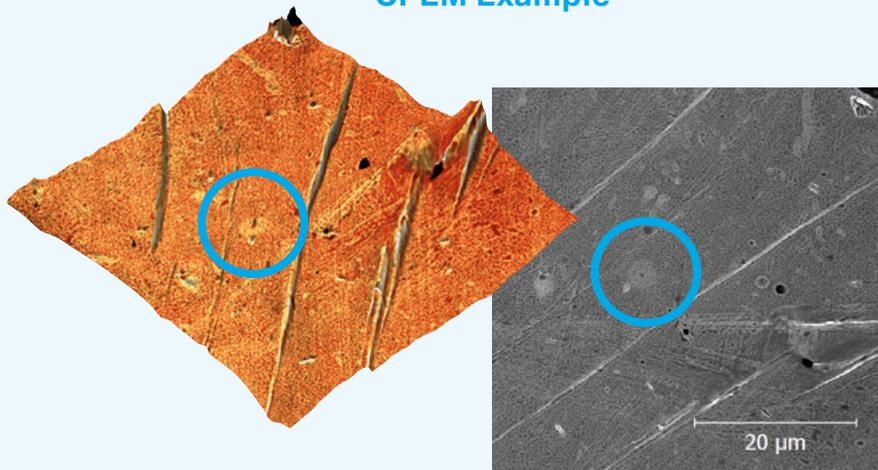
Comparison of a CPEM and an SEM image of fine-grained 9% Cr steel reinforced with fine yttrium oxide.
