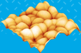
Textured PIN diode on glass substrate – solar cell, CPEM
