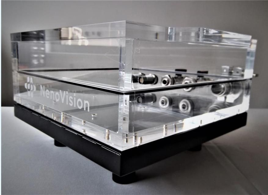
NenoCase™ is a new accessory for an Atomic Force Microscope (AFM) - LiteScope™. NenoCase™ is not only easy to use storage case but also opens new possibilities of usage LiteScope™ as a stand-alone device. It incorporates passive antivibration system to ensure high quality imaging outside the SEM chambers. NenoCase™ can be purged with different gases used for measurements under different atmospheres.
