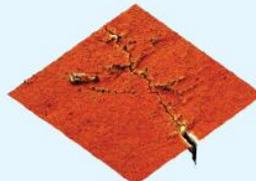
Crack propagation in metallic sample
